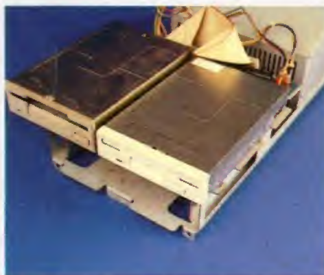
9 The XL drive at home. It may be a little whiter than the standard ones, but otherwise it looks just the same. Now 1.6 Mb disks are at your command.
